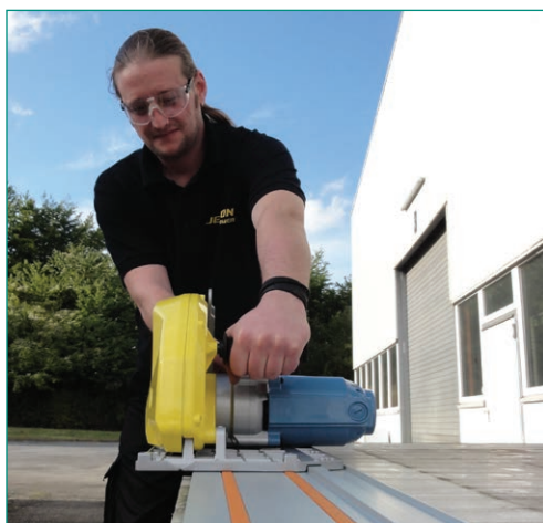
8320 SHDC Super Hand-Held Dry Cut Saw (608270 U) standard equipment includes a saw blade (P/N 608276).
