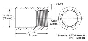
Operating Pressure: 2000 psi (13.8 MPa) [138 bar] Operating Temperature: 400 deg F (204 deg C)
