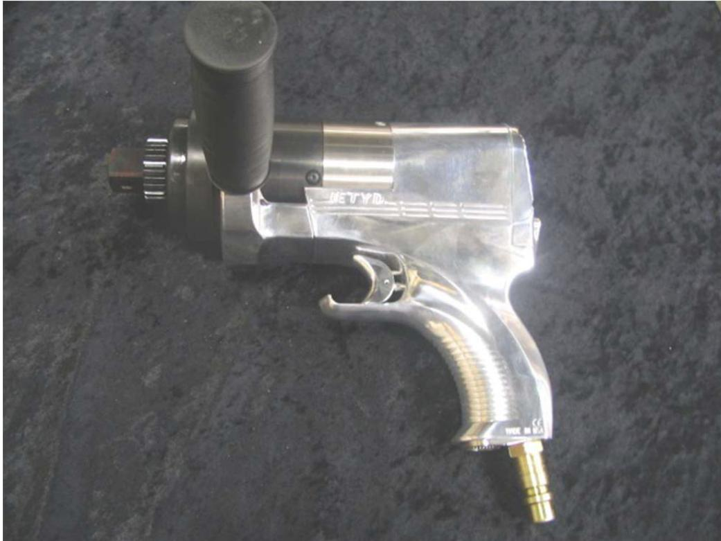
The handle shown above can be positioned on either side for right or left handed operation.
